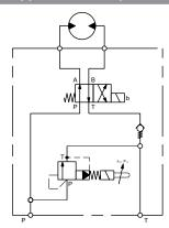
The valve is used to unload a pump to tank with a very low pressure drop. This results in less heating of the oil and therefore lower energy costs for the user.
