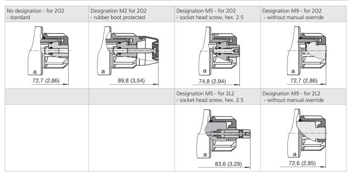
In case of solenoid malfunction or power failure, the spool of the valve can be shifted by manual override as long as the pressure in port 1 does not exceed 25 bar (363 PSI). For alternative manual overrides contact our technical support.
