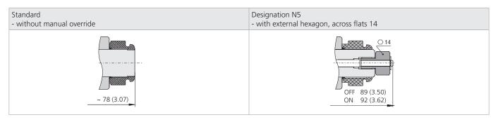
In case of solenoid malfunction or power failure, the spool of the valve can be shifted by manual override as long as the pressure in port T does not exceed 25 bar (363 PSI). For alternative manual overrides contact our technical support.
