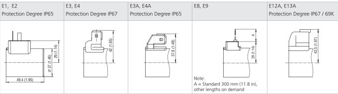
The indicated IP protection level is only achieved if the connector is properly mounted.
