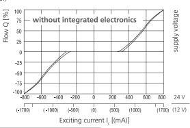
The coil current which initializes the flow through the proportional directional valve can differ due to the production tolerances about in a range of ± 6% of the limit current.
