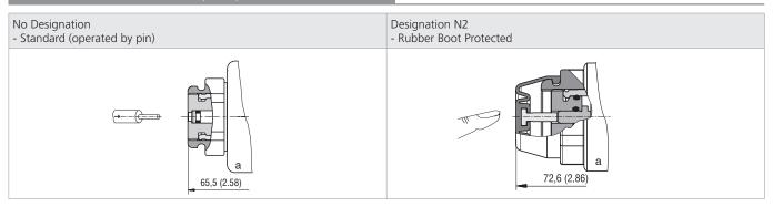
In case of solenoid malfunction or power failure, the spool of the valve can be shifted by manual override as long as the pressure in port T does not exceed 25 bar (363 PSI). For alternative manual overrides contact our technical support.
