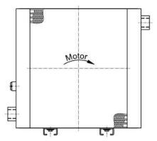
The oil inlet is on the left of the cooling matrix. The oil outlet is always on the opposite side.
