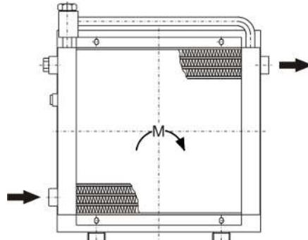
The oil inlet is always at the bottom left of the cooling battery. The second connection must be closed. The oil outlet is always on the opposite side.
